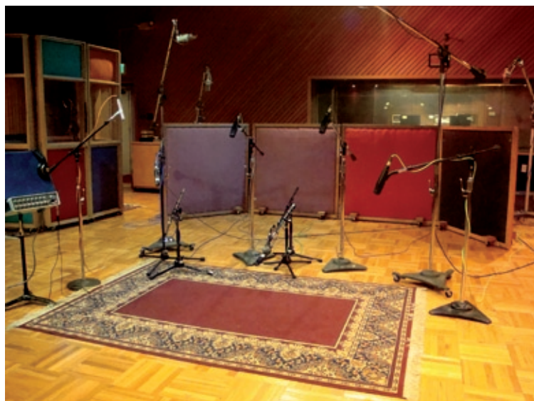
The drum mic setup in Fantasy's Studio A as it was for the recording of Dookie . This includes a pair of Telefunken tube 251s as overheads, an AKG D112 and a 421 for the kick, an SM57 on top of the snare and an AKG 451 underneath, Sennheiser MD421s for the toms (AKG 414s were also used) and Neumann M49s for the room.
