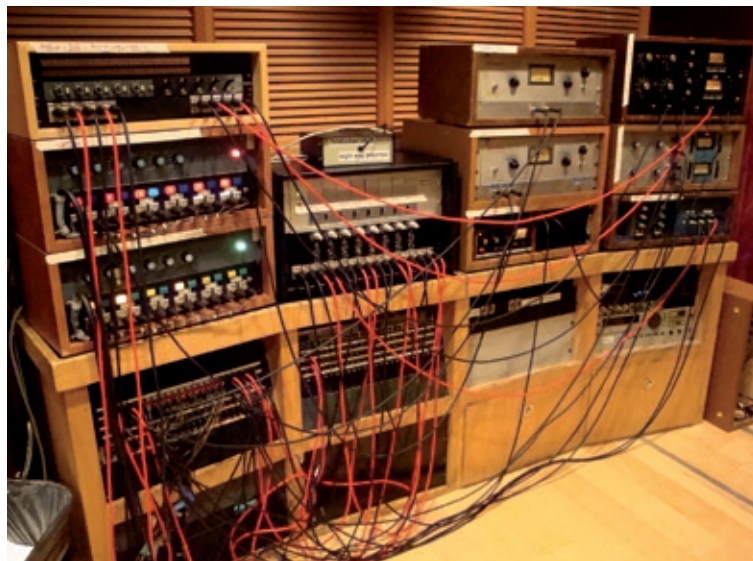
Outboard gear in Fantasy's Studio A control room. On the left-hand side is a rack of five Neve 8078 mic pres above two racks of six Neve 8078 mic pres. To the right of these is a rack of Telefunken 672 eight mic pres and, further to the right, a pair of Teletronix LA2A Tube Limiters, beneath which is a DBX 160 Compressor/Limiter. At the far right are a pair of Urei LN 'black face' 1176s and a pair of 'blue stripe' 1176s with an LN upgrade.
