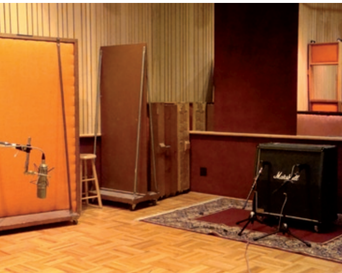
The mic setup for recording Billie Joe Armstrong's guitar overdubs in Fantasy's Studio B. The Marshall cab's two best cones are miked with an SM57 and a Sennheiser MD421. To the left you can see a U87 being used as a room mic.
