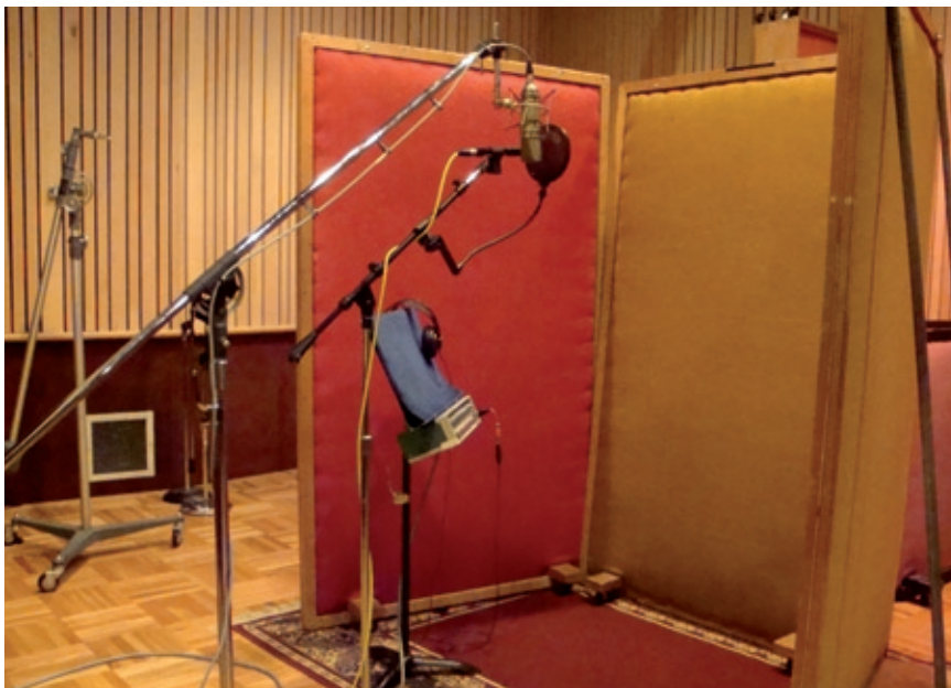
The Neumann U87 and Beyer M201 used for recording the vocal overdubs in Studio B.
